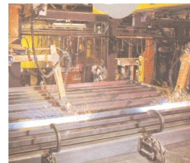
Modules are robotically welded
